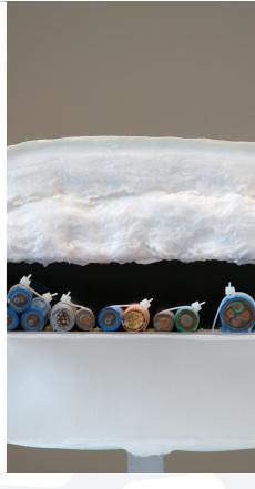
NuFCT 5111 is a flexible protection ensuring functionality of the protected cable tray for up to 2 hours under ISO It is adaptable to the environment. This protection is composed of mineral wool, refactory glue and a protective fabric. This complex has a thickness of 80 mm.
